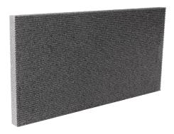
Unstressed insulation panel suitable for external thermal insulation systems, made of sintered expanded polystyrene (EPS) with the addition of graphite, with external grooved pattern to improve system impact resistance. TermoK8 A.R. Max 20 J and 60 J.
